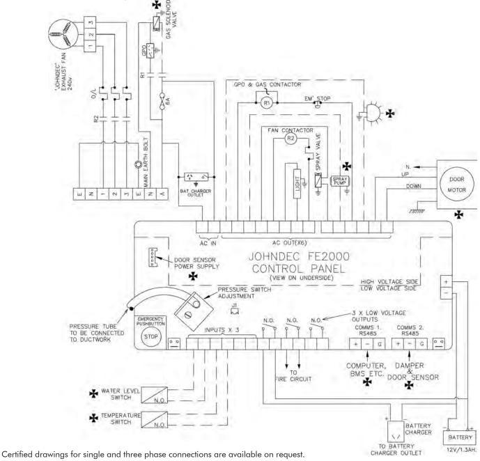
All of the above operating systems, switches, timers, relays etc are contained in the module measuring 250mm x 150mm x 70mm deep. The face of the panel is finished flush. All switches are of the touch design, except the mushroom headed emergency switch.
